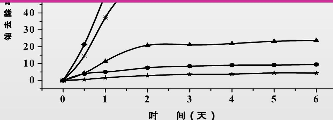
fig8 Different pH conditions, the impact of removal of uranium
