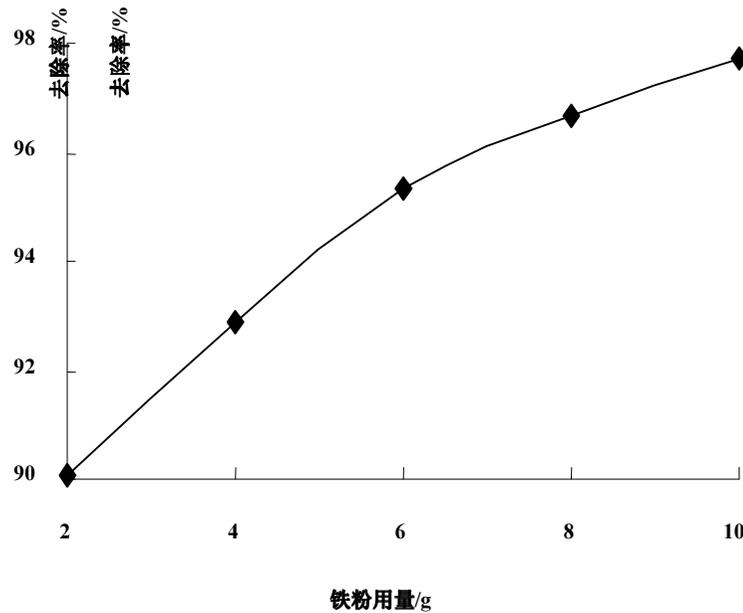
Fig.4 Effect of removal of U(VI) from aqueous solution by adsorption of ZVI
